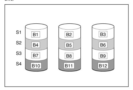
For data in the logical drive to be readable, the data block sequence must be the same in every stripe. This sequencing process is performed by the array controller, which sends the data blocks to the drive write heads in the correct order.
