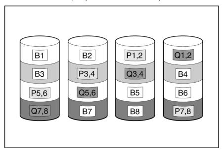
This method is most useful when data loss is unacceptable but cost is also an important factor. The probability that data loss will occur when an array is configured with RAID 6 (ADG) is less than it would be if it were configured with RAID 5.
