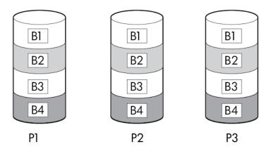
When the array has more than three physical drives, drives are mirrored in trios, and the fault-tolerance method is known as RAID 10 (ADM). If a physical drive fails, the remaining two drives in the mirrored trio can still provide all the necessary data. Several drives in the array can fail without incurring data loss, as
