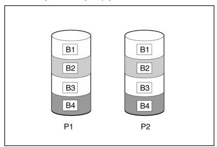
When the array has more than two physical drives, drives are mirrored in pairs, and the fault-tolerance method is known as RAID 1+0 or RAID 10. If a physical drive fails, the remaining drive in the mirrored pair can still provide all the necessary data. Several drives in the array can fail without incurring data loss, as long as no two failed drives belong to the same mirrored pair. The total drive count must increment by 2 drives.
