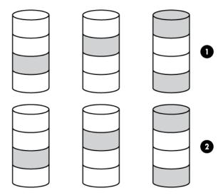
For any given number of hard drives, data loss is least likely to occur when the drives are arranged into the configuration that has the largest possible number of parity groups. For example, four parity groups of three drives are more secure than three parity groups of four drives. However, less data can be stored on the array with the larger number of parity groups.
