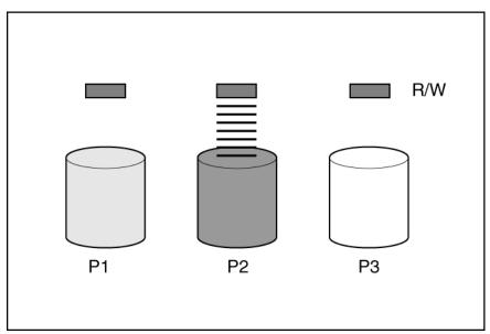
With an array controller installed in the system, the capacity of several physical drives can be combined into one or more virtual units called **logical drives** (also called **logical volumes** and denoted by Ln in the figures in this section). Then, the read/write heads of all the constituent physical drives are active simultaneously, reducing the total time required for data transfer.
